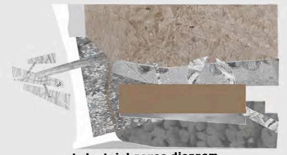
industrial reuse diagram REUSE of old foundations on site for hillside seating debris for pathways, retain existing concrete slab SUBTERRANEAN REUSE hillside from reclaimed fill
